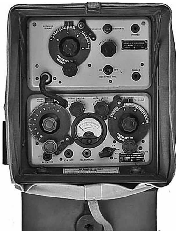
WS48 MkI* set with canvas rain cover, and battery compartment underneath. The front panels were bright green to aid reading of labels in low light.
