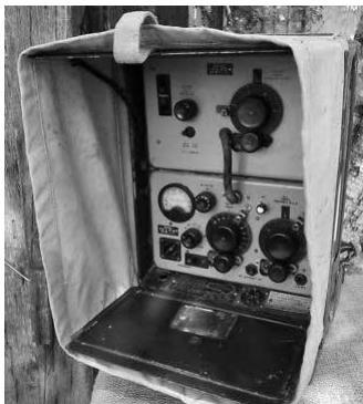
WS18 the British precursor to the WS48. Front panels were either grey or black.
